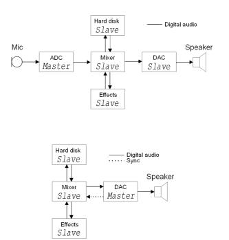
Figure 11 Digital studio setup with an ADC or DAC as master.
