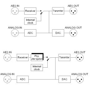
Figure 3 Clock circuit in a conventional design and in System 6000
