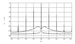
Figure 9 Zoomed (frq. only) version of Figure 8 (lower) plus the same level of jitter applied to a conventional design (upper).
