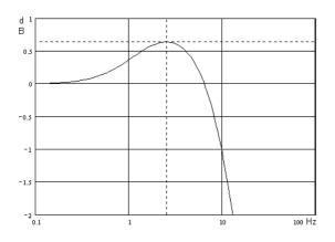
Figure 5 Zoomed picture of the jitter rejection filter.
