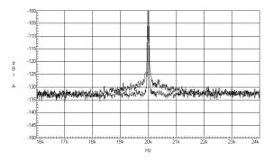
Figure 7 Zoomed version (both frq. and level) of Figure 6 plus System 6000 in slave mode.
