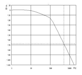
Figure 4 Jitter rejection filter (4'Th order filter)
